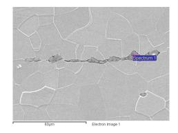
**Fig.4.** Inclusions broken into small pieces with a long chain.
