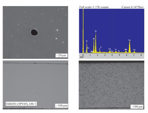
Fig.6. Analyses of steel coils with control of f[O] prior to addition of ferrosilicon.
