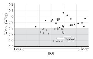
**Fig.7.** Effect of f[O] prior to addition of ferrosilicon on core loss.
