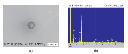
Fig.1. Inclusion shape and composition of 50CS1300 with low core loss.
